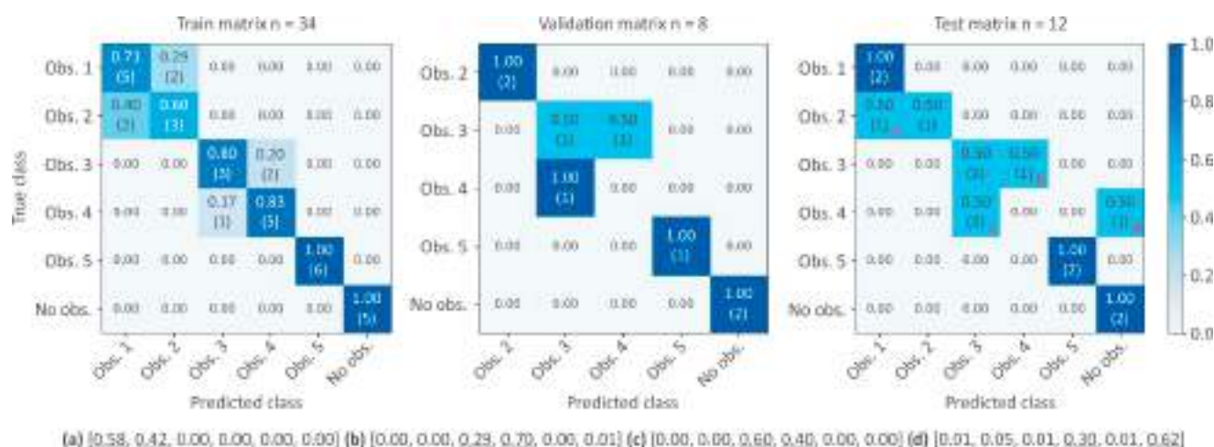
Figure 7. Confusion matrix for training, validation, and test datasets using three nodes. Misclassifications in the test dataset correspond to obstruction in the second cross-wall notch (a), obstruction in third cross-wall orifice (b), obstruction in the fourth cross-wall notch (c), and obstruction in the fourth cross-wall orifice (d) (class probabilities of misclassifications are indicated at the bottom of the picture).
