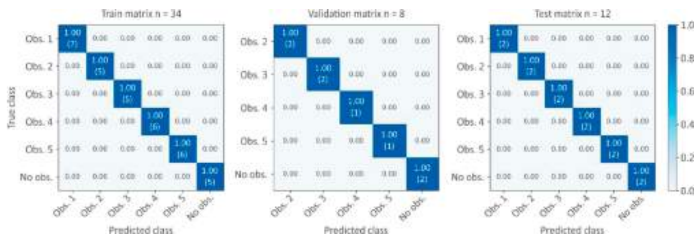
Figure 6. Confusion matrix for training, validation, and test datasets (42 simulated scenarios; 12 measured scenarios) using five nodes, i.e., a node per pool (obs. = obstruction; n = number of scenarios). The numbers in the matrix correspond to percentages (sum by row = 1.00) while the numbers between parentheses correspond to the number of scenarios.
