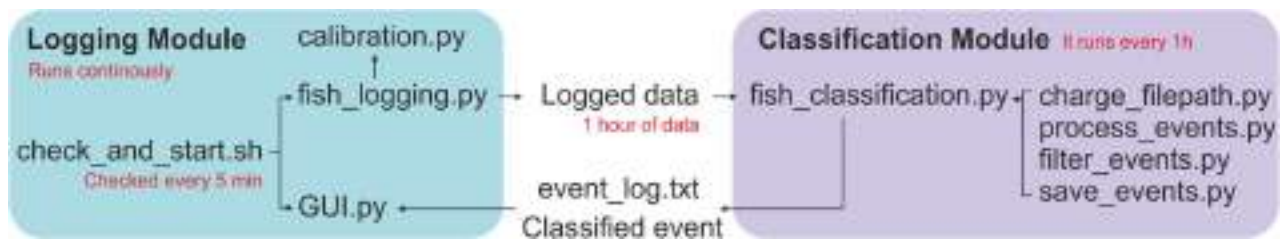
Figure 5. Diagram of the Fish Tracker software architecture. The logging module runs continuously, saving hourly binary data and performing real-time calibration. The classification module, executed every hour, processes the logged data to extract and validate fish passage events using a series of interconnected scripts.
