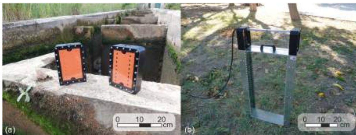
Figure 3. Two Fish Tracker prototypes. (a) The Fish Tracker Mini, an initial prototype with 8 IR photodetectors per array, which was used for early functional testing and alignment verification. (b) The final Fish Tracker system (full version), featuring 40 IR photodetectors per array and full-scale structural dimensions, enclosed in waterproof aluminum housing for field deployment.
