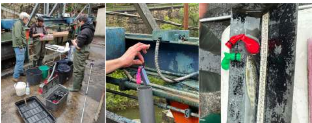
Figure 2. Tagging and injection with balloon tags. (Left) equipment overview. (Center) Injection pipe with pressure tag ready for release. (Right) Salmon smolt tagged with two balloon tags.
